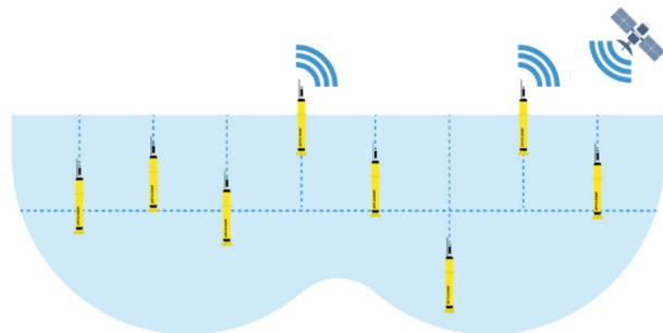
Figure 20: ONE ARGO: Standard Argo profiling floats (temperature, salinity) in upper 2,000m with Biogeochemical Argo and Deep Argo (6,000m) being added.
