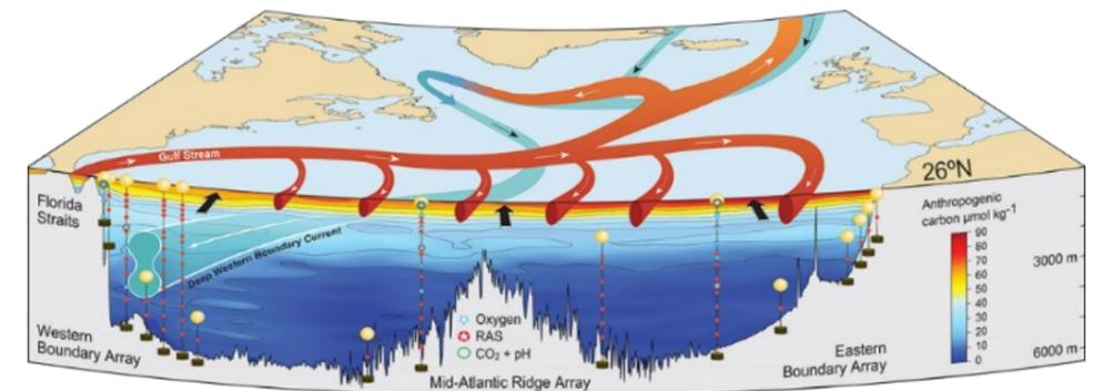
Figure 16: Schematic of the Atlantic Meridional Overturning Circulation (AMOC) with concentrations of anthropogenic carbon concentrations at 24.5°N in 2010. ABC will deploy biogeochemical sensors (oxygen, pCO<sub>2</sub>, pH) and remote access sampling (RAS) on some of the RAPID moorings, as indicated in the figure. Credit: NOC/P. Brown & V. Byfield.
