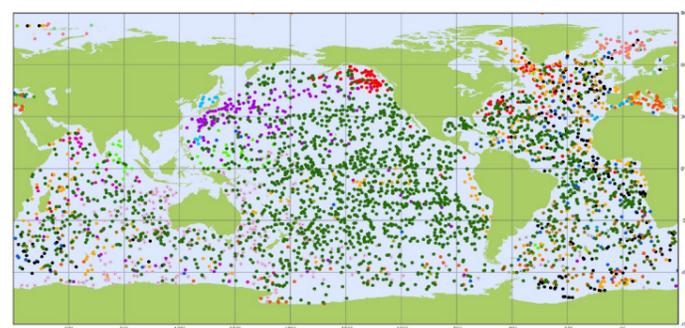
Figure 21: The global array of Argo profiling floats – the majority are standard Argo (temperature and salinity to 2,000m depth) with biogeochemical floats (currently about 300) and Deep Argo (very few) being added/substituted. Credit: Argo (2023)
