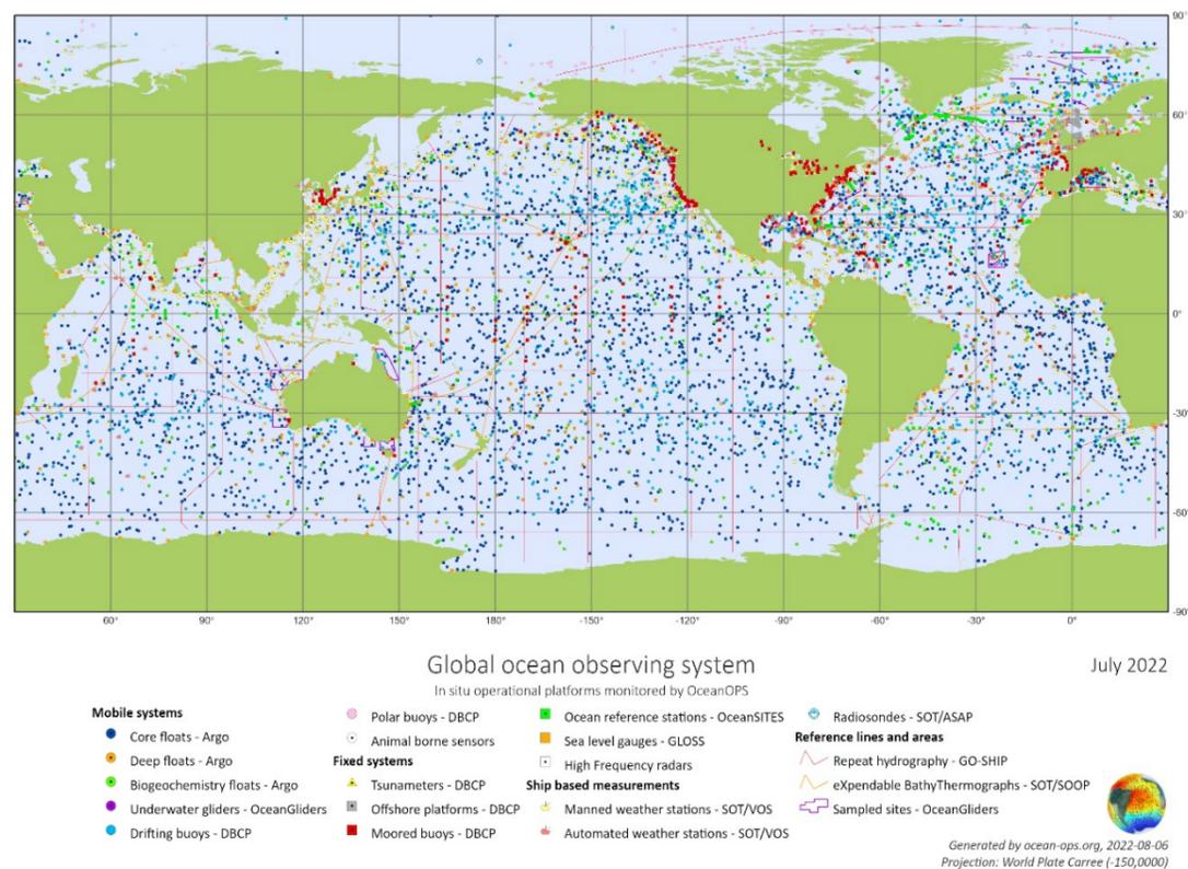
Figure 7: The Global Ocean Observing System is a 'system of systems' and its major component systems are shown. (Credit: ocean-ops.org 22-08-6)
