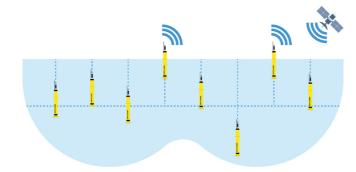
Figure 20: ONE ARGO: Standard Argo profiling floats (temperature, salinity) in upper 2,000m with Biogeochemical Argo and Deep Argo (6,000m) being added.
