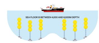
Figure 15: AMOC: Atlantic Meridional Overturning Circulation - trans-Atlantic (26°N) moored buoy array serviced by research ship.
