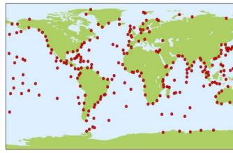
Figure 31: The GLOSS Core Network of coastal and oceanic island tide gauges - the UK contributions are around UK coast (Environment Agency) and South Atlantic oceanic islands and Antarctica (UKRI-NERC) Credit: PSMSL
